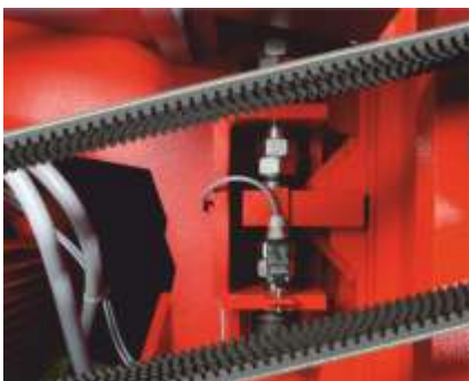
Safety package with gear limit switch and reverse counter
