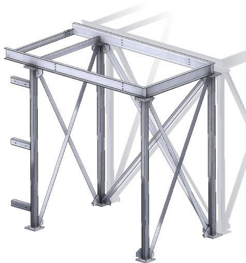
6 YARD BIN STRUCTURE
